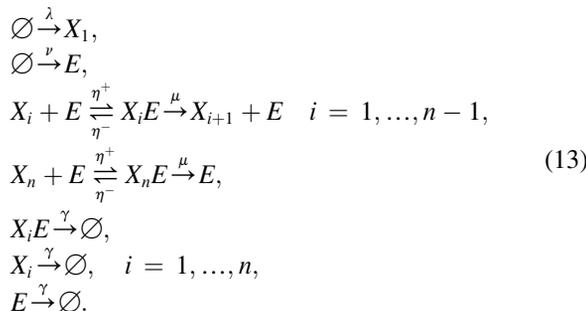
The mass-action model of adaptive queueing in a serial network with the continuous variables for ensemble averages  $\bar{Q}_i$  and  $\bar{L}$  is:
