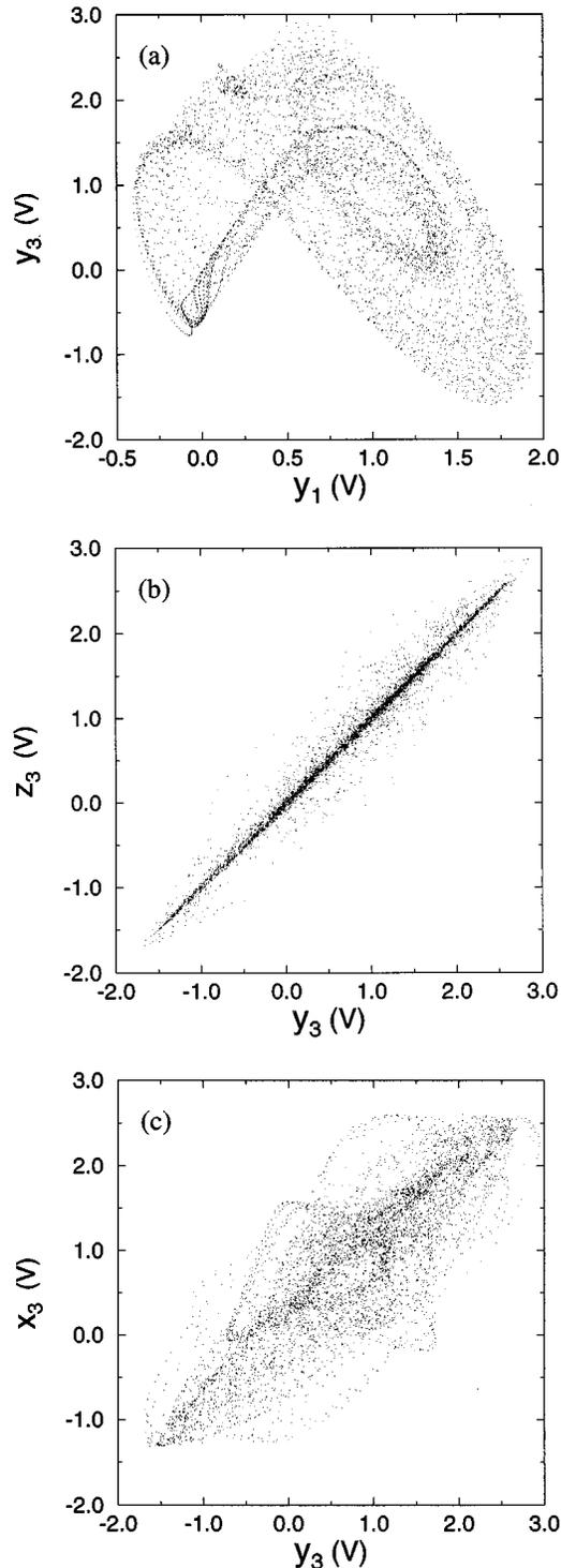
FIG. 5. Experimentally measured aspects of the unsynchronized chaotic attractor in the setup shown in Fig. 2. The coupling resistor was set at  $R_c = 731 \Omega$ . (a) is the projection of the attractor onto the  $(y_1, y_3)$  plane, (b) is the projection of the attractor onto the  $(y_3, z_3)$  plane, and (c) is the projection of the attractor onto the  $(y_3, x_3)$  plane. From (b) we conclude that the systems are not synchronized.
