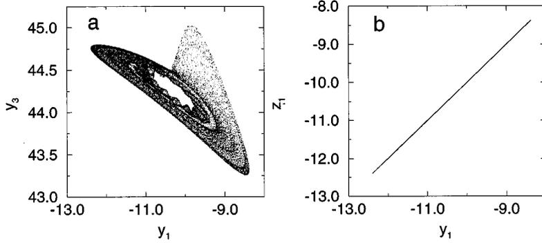
FIG. 1. Projections of synchronized attractors in the coupled Rössler and Lorenz systems. The coupling parameter is  $g = 10$  and the systems are coupled as indicated in the text. The Rössler system acts as the drive and the Lorenz system is the response. The projection of the response system onto the  $(y_1, y_3)$  plane is shown in (a). At this value of  $g$  the systems are synchronized. We can see this in the projection of the same attractor onto the  $(y_1, z_1)$  plane in (b).
