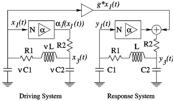
FIG. 1. The sketch of the circuit diagram for the experimental study of chaos synchronization with frequency ratio 2:1. The frequency ratio is controlled by the multiplier  $\nu$  used to select the values of the inductors and capacitors in the drive and response circuits.
