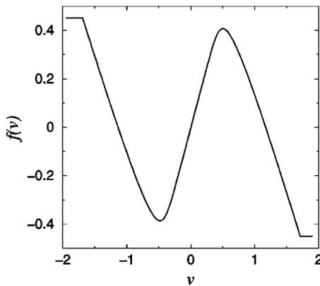
FIG. 2. The shape of the nonlinear function  $f(\ )$  measured in the experimental setup.
